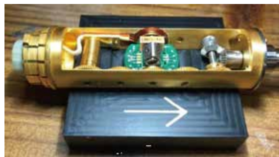
Fig. 2 Photograph of a miniature pressure cell placed on the horizontal rotator for PPMS
